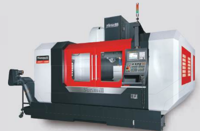
JMV-1600 X/Y/Z travel: 1600x850x750mm
